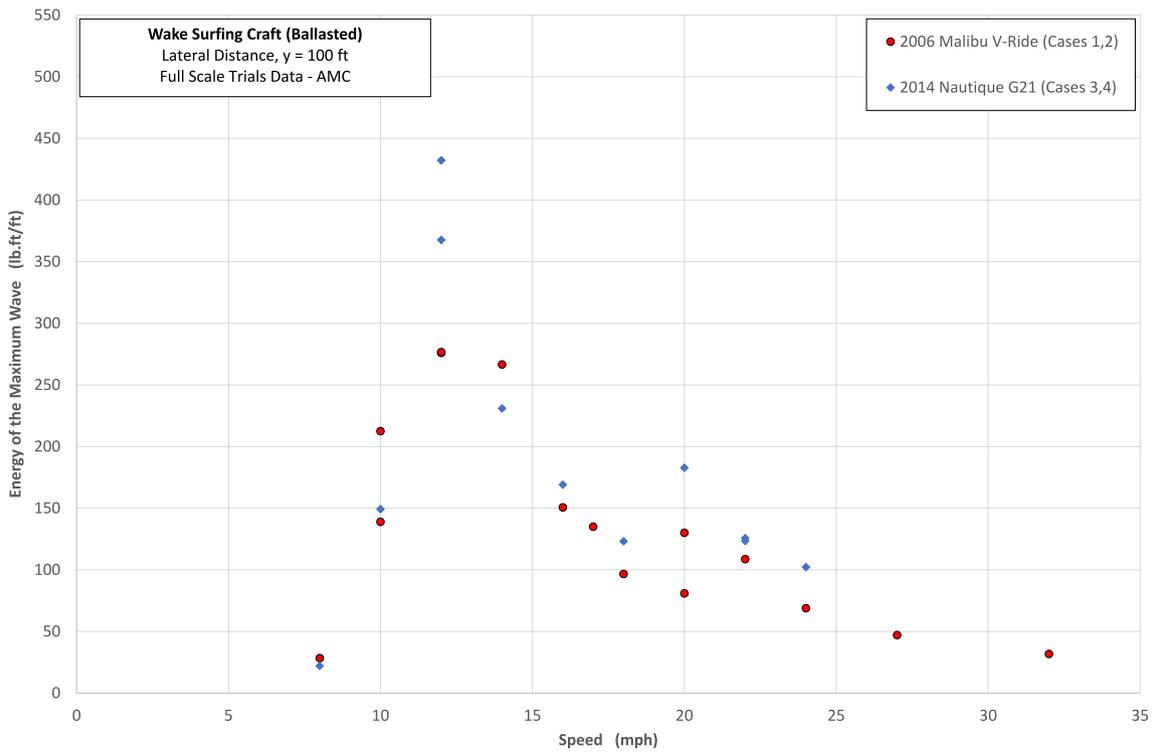
**FIGURE 6** | Energy of the maximum wave as a function of vessel speed for two wake boats: 2006 Malibu V-Ride (Cases 1 and 2) and 2014 Nautique G21 (Cases 3 and 4) at a lateral distance of 100 ft. Similar to the wave height and period, the peak wave energy occurs around 12 mph. [Color figure can be viewed at [wileyonlinelibrary.com](https://onlinelibrary.wiley.com)]
