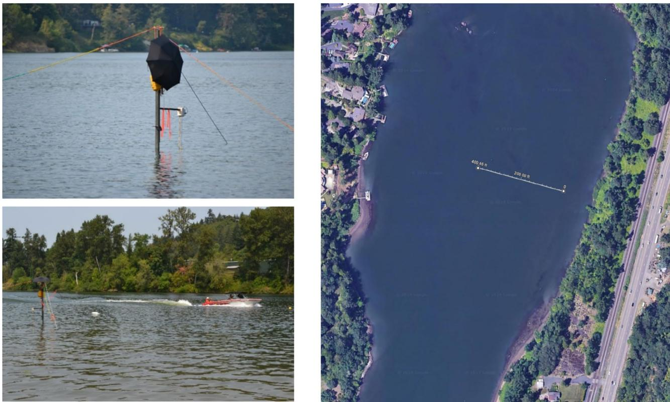
**FIGURE 3** | Right—Location of the test site on the Willamette River. The water depth at the wave sensor was 15 ft and approximately 40 ft at each of the vessel track paths (100, 200, 300, 400 ft from the sensor at  $y=0$  ft). Top left—Wave sensor attached to a rigid vertical pole. Bottom left—Test vessel passing the wave sensor. [Color figure can be viewed at [wileyonlinelibrary.com](https://onlinelibrary.wiley.com)]
