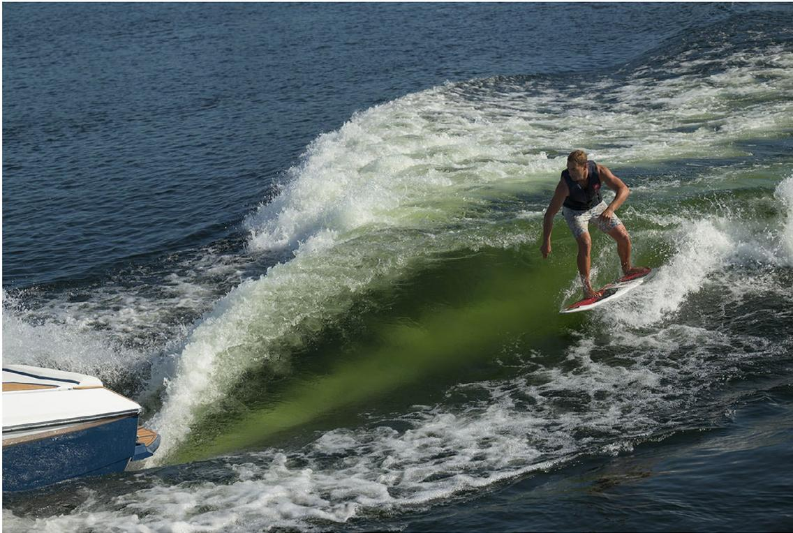
**FIGURE 1** | Wakesurfing in the enhanced and tuned wave a short distance aft of the transom of a typical wake boat. *Note:* The asymmetry of the wake and the long, high, clean, and steep wave face (Nautique Boats 2024). [Color figure can be viewed at [wileyonlinelibrary.com](https://onlinelibrary.wiley.com/doi/10.1002/rra.4438)]
