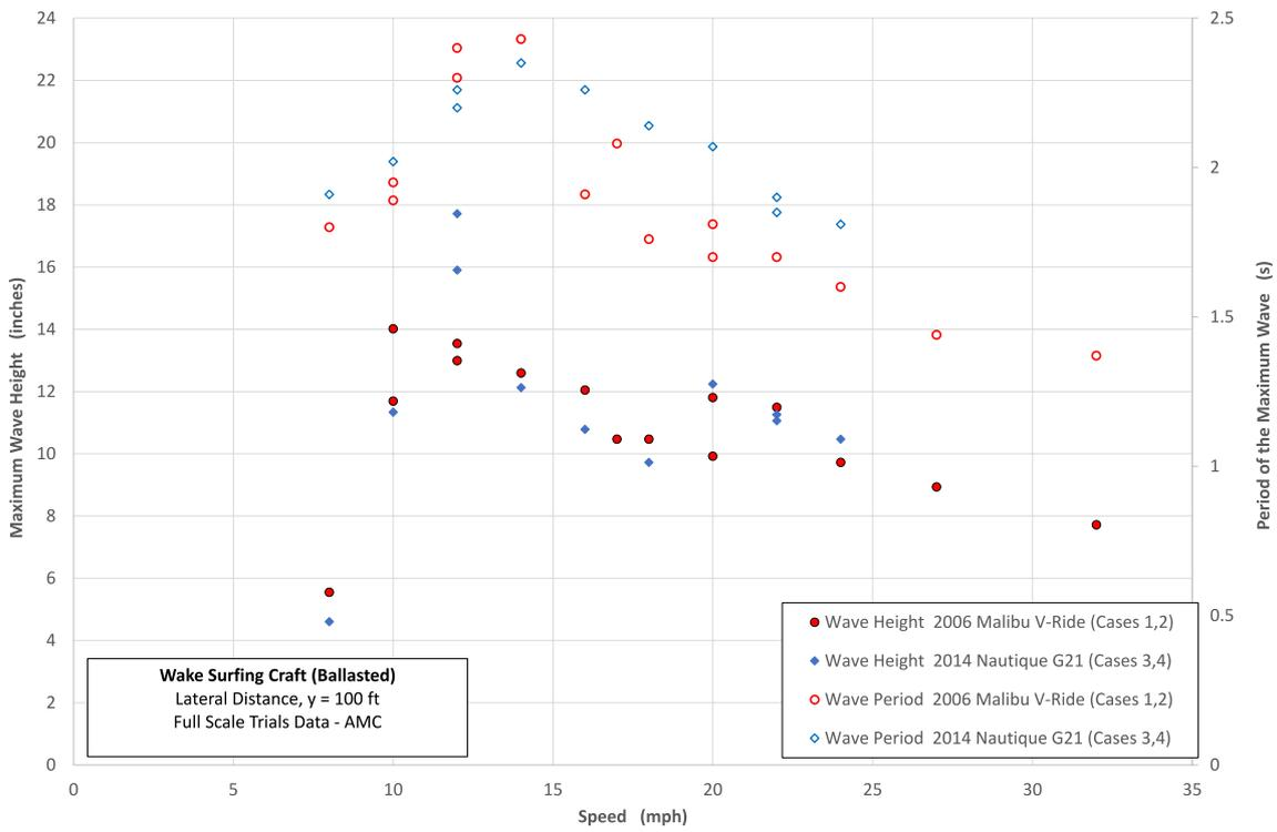
**FIGURE 5** | Maximum wave height and period as a function of vessel speed for two wake boats: 2006 Malibu V-Ride (Cases 1 and 2) and 2014 Nautique G21 (Cases 3 and 4) at a lateral distance of 100 ft. The peak wave height occurs around 10–12 mph and the peak wave period around 12–14 mph. [Color figure can be viewed at [wileyonlinelibrary.com](https://onlinelibrary.wiley.com)]
