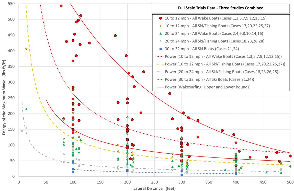
**FIGURE 11** | Energy of the maximum wave as a function of lateral distance for each of the three nominal speed ranges (all studies combined): 10–12 mph (red), 20–24 mph (green), and 30–32 mph (blue). Boat categories (wake or ski/fishing) are also identified. Power trendlines are included to assist interpretation. [Color figure can be viewed at [wileyonlinelibrary.com](https://onlinelibrary.wiley.com)]
