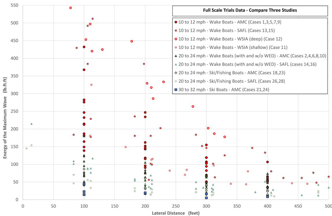
**FIGURE 9** | Energy of the maximum wave as a function of lateral distance for each of the three nominal speed ranges: 10–12 mph (red), 20–24 mph (green), and 30–32 mph (blue). Where appropriate, the data have been sub-categorized into each of the three studies (AMC, WSIA, and SAFL). [Color figure can be viewed at [wileyonlinelibrary.com](https://onlinelibrary.wiley.com)]
