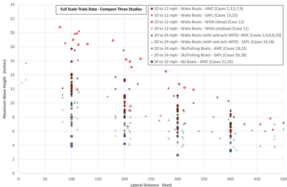
**FIGURE 7** | Maximum wave height as a function of lateral distance for each of the three nominal speed ranges: 10–12 mph (red), 20–24 mph (green), and 30–32 mph (blue). Where appropriate, the data have been sub-categorized into each of the three studies (AMC, WSIA, and SAFL). [Color figure can be viewed at [wileyonlinelibrary.com](https://onlinelibrary.wiley.com)]
