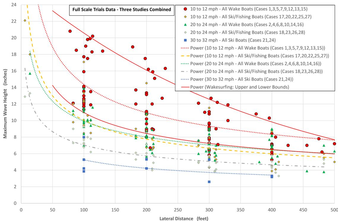
**FIGURE 10** | Maximum wave height as a function of lateral distance for each of the three nominal speed ranges (all studies combined): 10–12 mph (red), 20–24 mph (green), and 30–32 mph (blue). Boat categories (wake or ski/fishing) are also identified. Power trendlines are included to assist interpretation. [Color figure can be viewed at [wileyonlinelibrary.com](https://onlinelibrary.wiley.com)]
