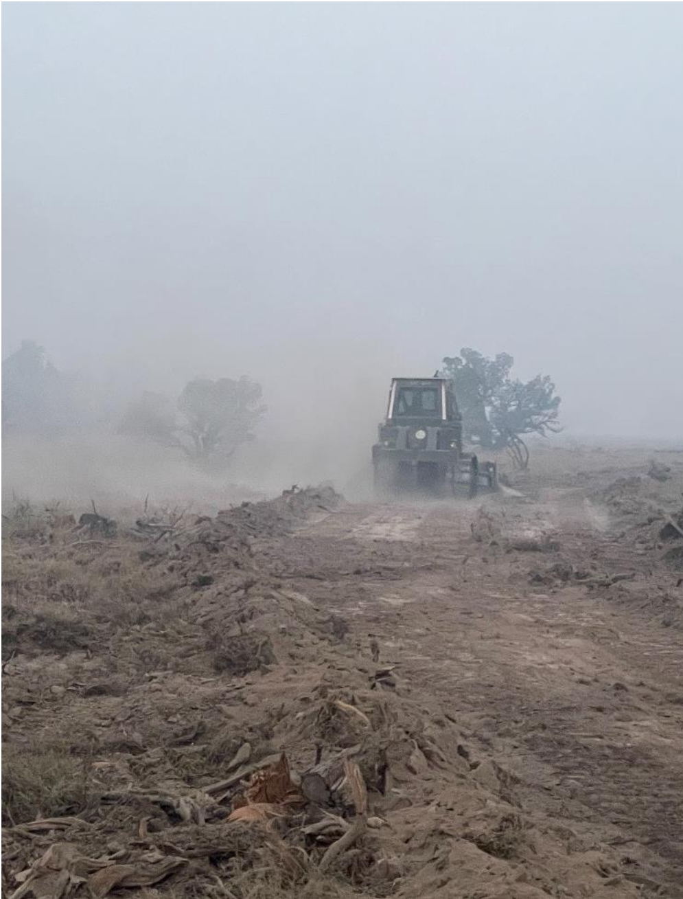
July 16, 2024. 5:00 am. Building fire containment line with our dozer. We have built 6 miles of line, met up with a Forest Service dozer on the other end, and are heading back to the beginning doubling up on the line width.
