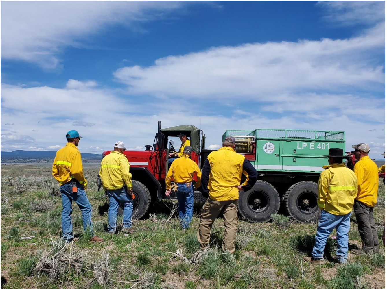
Annual fire training using one of our fire engines that was built on a used military chassis.
