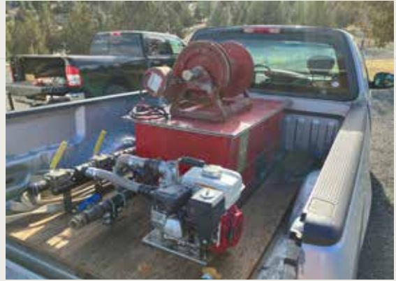
A slip on tank that fits in truck bed. Filled with water it provides another water source for dousing fires.
