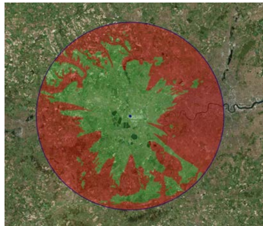
Figure 3: typical radar viewshed model (red = not visible; green = visible)
