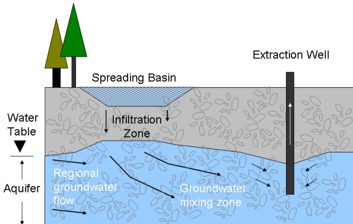
**Figure 3. In a typical spreading basin project, water infiltrates through shallow basins or canals. Withdrawal occurs down gradient through a well or the water discharges to the surface and augments stream flow.**
