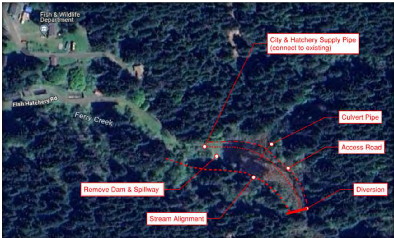
Figure 3.2 – Bandon – Proposed Ferry Creek Dam Relocation
