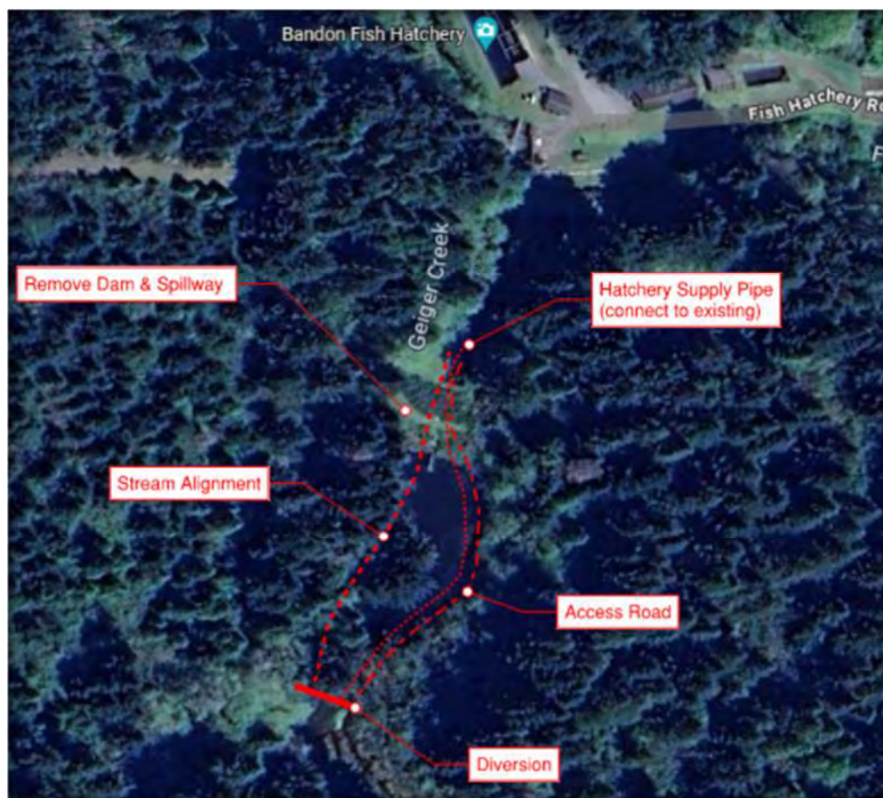
Figure 3.1 – Bandon – Proposed Geiger Creek Dam Relocation
