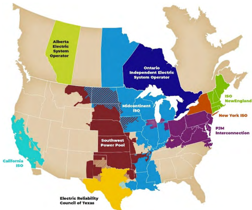
Figure 3: Map of Regional Transmission Organizations and Independent System Operators in the U.S. and Canada 27
