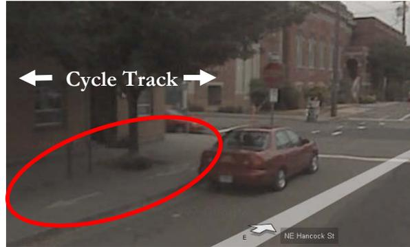
Figure 25. Contraflow cycle track on NE Hancock Street in Portland, OR
