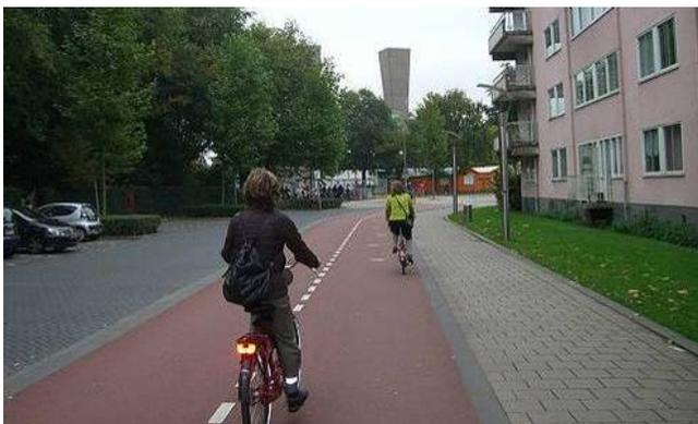
Figure 18. Two-way cycle track with dividing line
