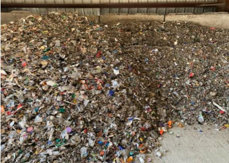
*Picture of typical Commingled Single Stream Recycled “Glass” - as delivered from a Materials Recovery Facility for processing. Intensity of secondary processing (additional sorting and cleaning prior to meeting furnace-ready specifications) depends on contamination levels. This also impacts MRF “market price” due to hauling higher percentages of residual material that then must be landfilled.*
