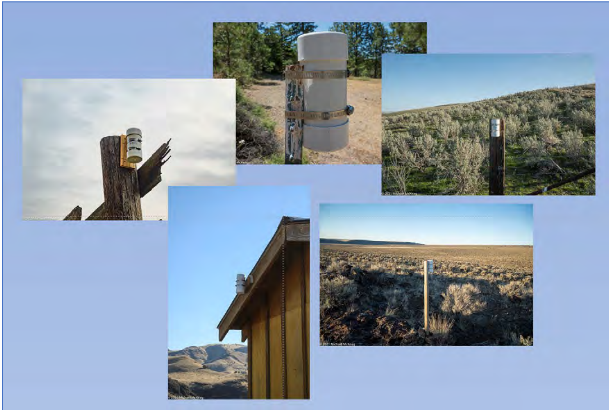
Figure 2. Examples of SQMs installed at sites in Oregon. The meter resides inside a weatherproof case and points vertically toward the sky.
