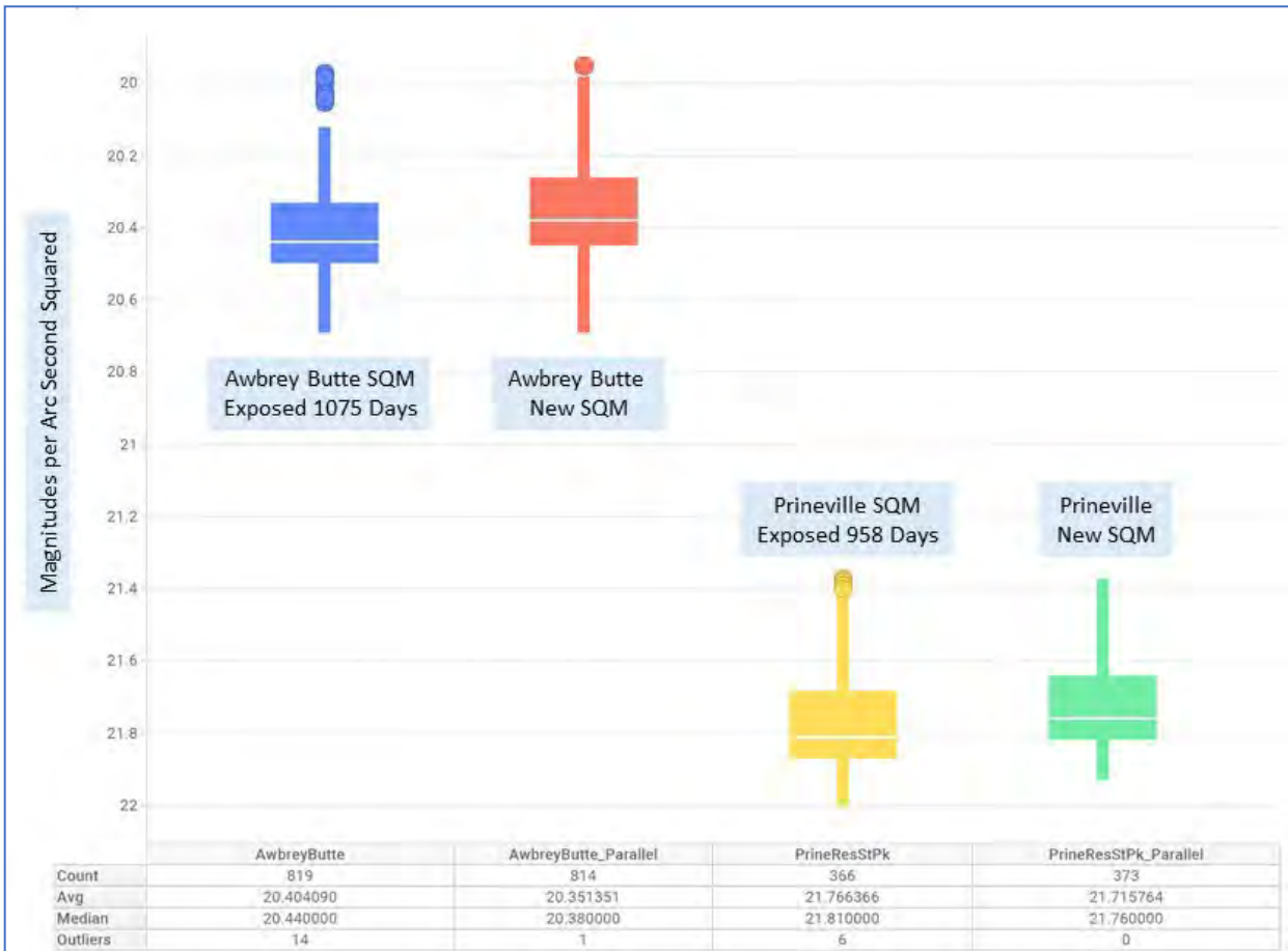
Figure D2. Box plot comparing data recorded by the two sets of parallel-running SQMs. In both cases, the older SQMs recorded slightly darker skies on average.
