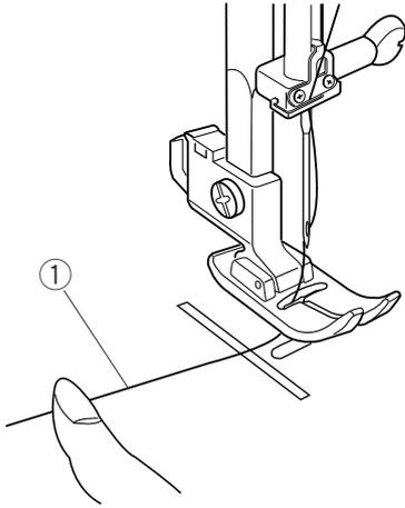
1 Raise the presser foot and hold the needle thread lightly with your left hand.
