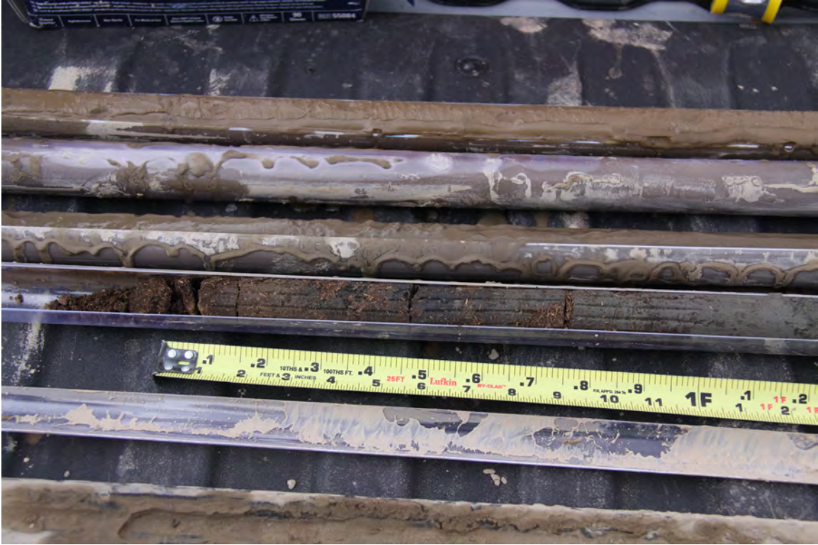
Image: Sample from DBD Compost area with 1' of compacted manure
