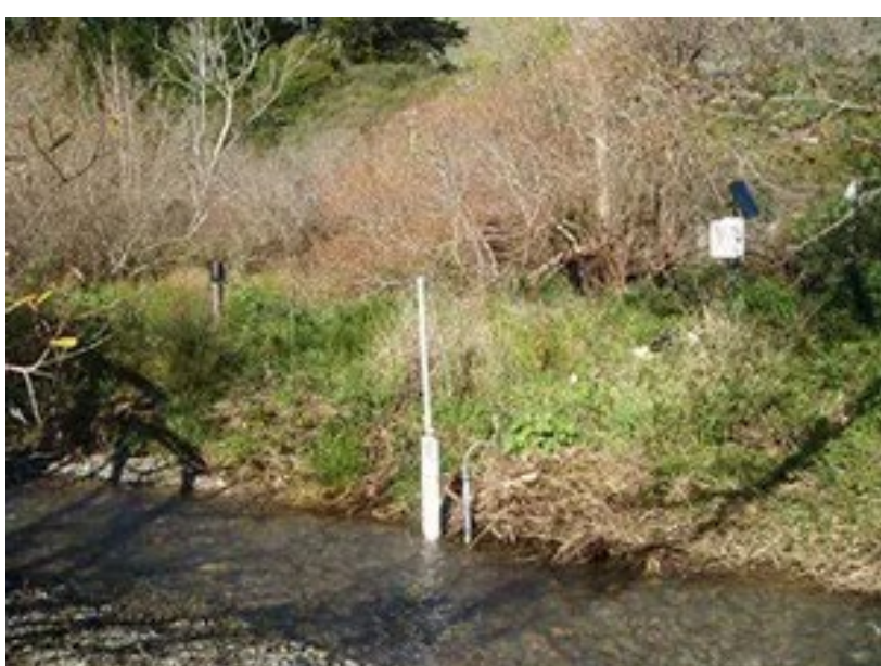
Acquiring a stream gauge for Lookingglass Creek to measure project effectiveness for a habitat restoration/floodplain reconnection project set to be implemented by Confederated Tribes of the Umatilla Indian Reservation (CTUIR) in 2025.
