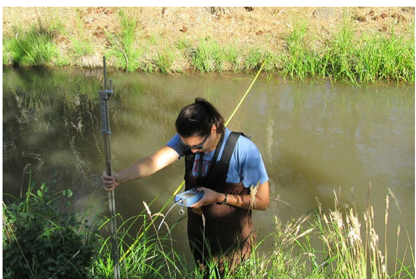
Developing instream flow targets using field-based Instream Flow Incremental Methodology in conjunction with desktop-based hydrologic analyses for the Upper Grande Ronde River. Results will aid in flow restoration and water planning efforts (fall 2022).
