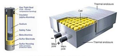
Sodium-Sulfur (NaS) Batteries
