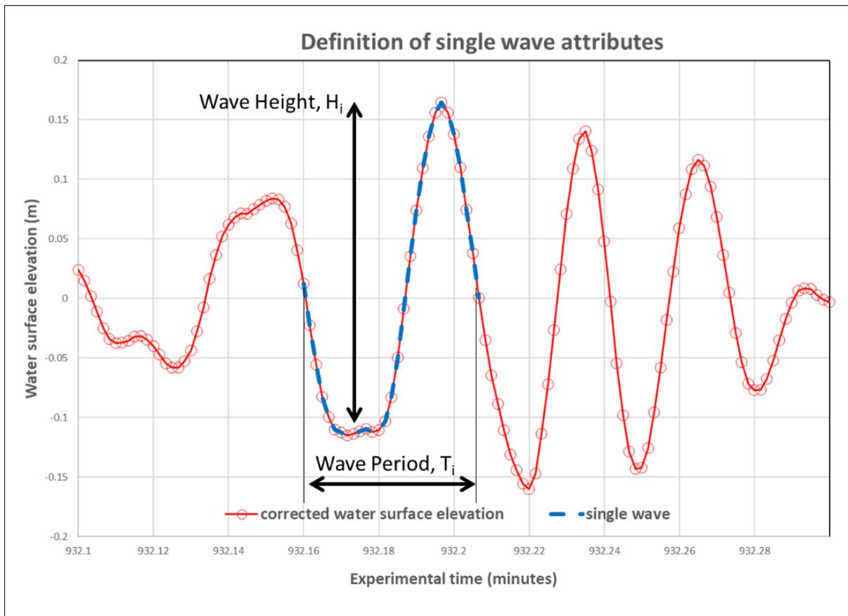
Figure 11. Definitions of zero-crossing down (blue dashed line) as well as wave characteristics of wave height,  $H_i$  and wave period  $T_i$ , where subscript  $i$  is an integer representing the sequential number of a wave within the packet.
