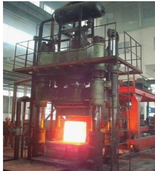
Full scale forging Ingot approximately 4ft x 3ft, material cost greater than $50,000
