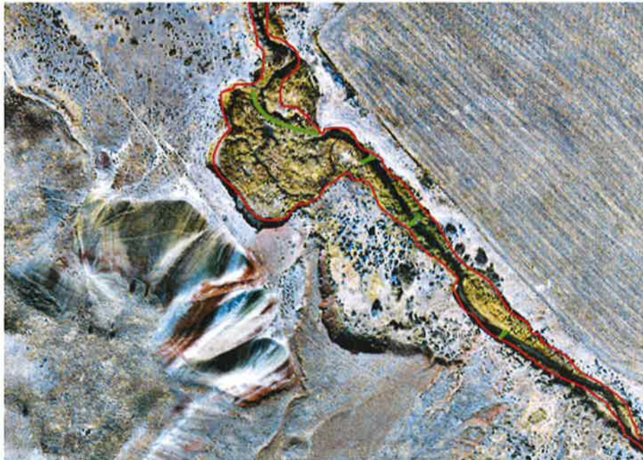
Figure 7. An aerial orthophotograph of beaver dams (green lines) and riparian vegetation adjacent to Painted Hills National Monument. The red line outlines the stream-adjacent area within 0.5 m elevation of the existing stream channel. The large, downstream beaver dam has aggraded the stream bed over 1 m in the past 6 years, raising the water table and allowing riparian vegetation to rapidly expand onto a formerly abandoned terrace such as the one immediately upstream.
