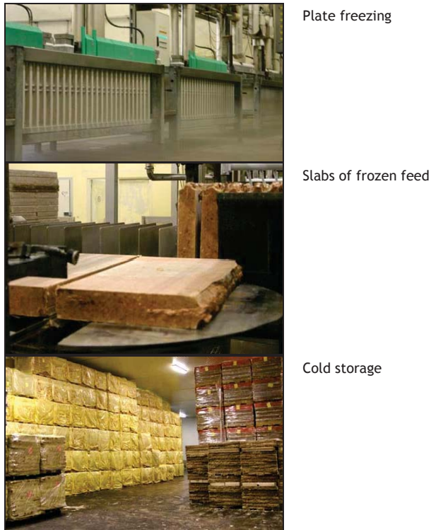
Figure 5 Feed production: plate freezing and storage
