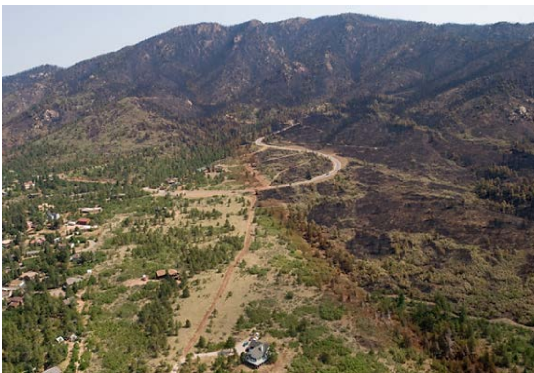
The community on the left was protected from the 2012 Waldo Canyon Fire in Colorado, by the area of reduced fuels in the middle ground—between the subdivision and the wildlands. Photo credit: Kari Greer, National Interagency Fire Center.
