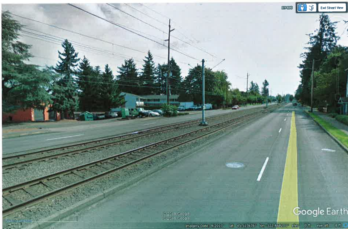
Figure 2. SE 193rd & Burnside fatality location showing no safe space between traffic lane and trackway
