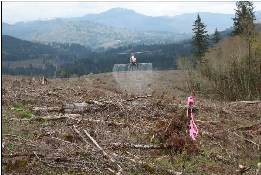
Figure 1 – Nozzle technology creates large droplet size which produce little drift.
