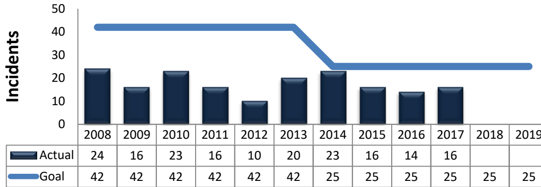
Derailment Incidents - Number of derailments caused by human error, track, or equipment
