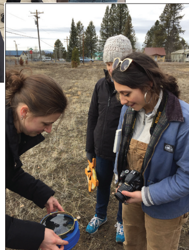
Passive Heating students using a Pathfinder to analyze solar access in La Pine.
