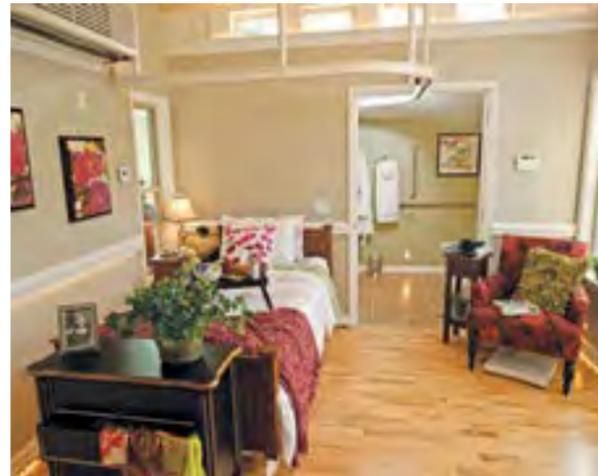
The MEDCottage has room for a bed, living area, kitchenette and ADA-accessible bathroom. Soft flooring helps cushion the impact of falls. (The company claims you can drop an egg from 18 inches without it cracking.) A ceiling track rail is available for a mobility lift if one is needed.
