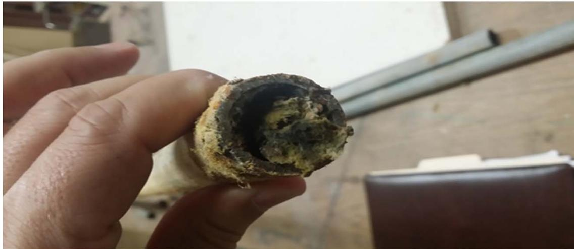
Picture of galvanized, deteriorated, and corroded pipe from Douglas County courthouse
