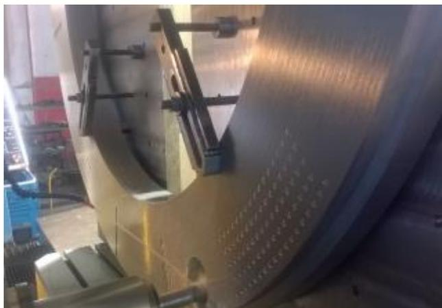
Machining of Tube Sheet
