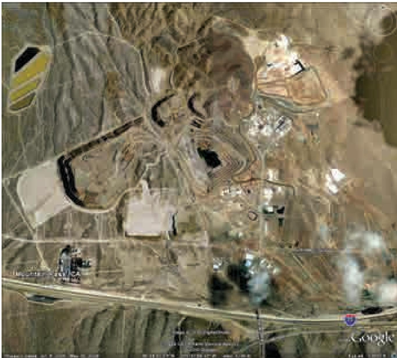
**Figure 6.** Google Earth image of the Mountain Pass mining district, California. Molycorp’s open pit mine—inactive since 2002—is at the center of this view; the pit covers about 55 acres (22 hectares) and is about 400 ft (122 m) deep. (Image used with permission of Google.)
