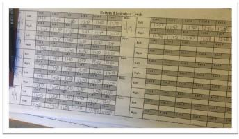
Weekly generator tests are needed, on a Monday not a Sunday. This requires opening the battery cell for a hydrometer test.
