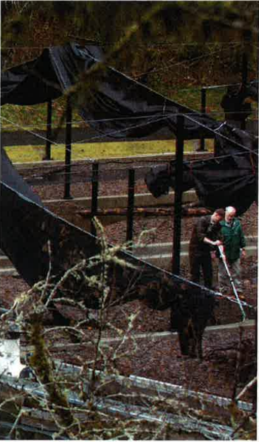
Water from Fall Creek flows into four parallel experimental channels, protected by netting from fish-eating birds.
