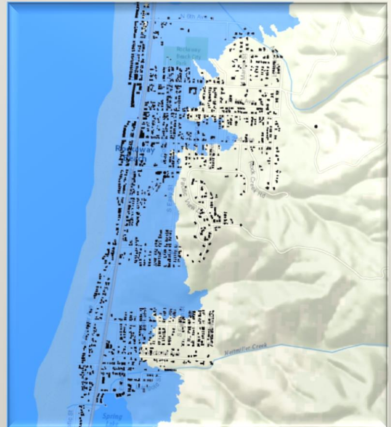
Modeled Cascadia tsunami inundation at Rockaway Beach
