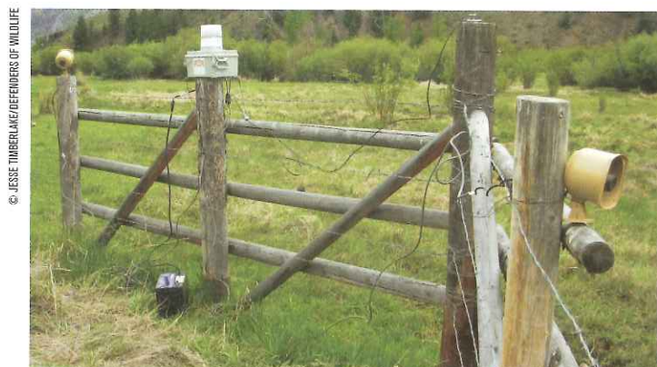
The radio-activated guard system—RAG box for short—affixed to this fence consists of loudspeakers and a battery-powered computer housed in a metal box.
